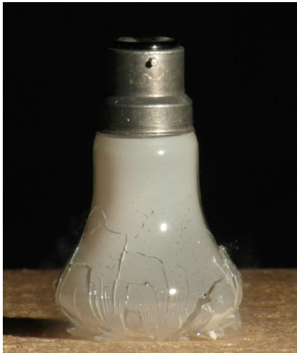
Glass breaking – using sound trigger
